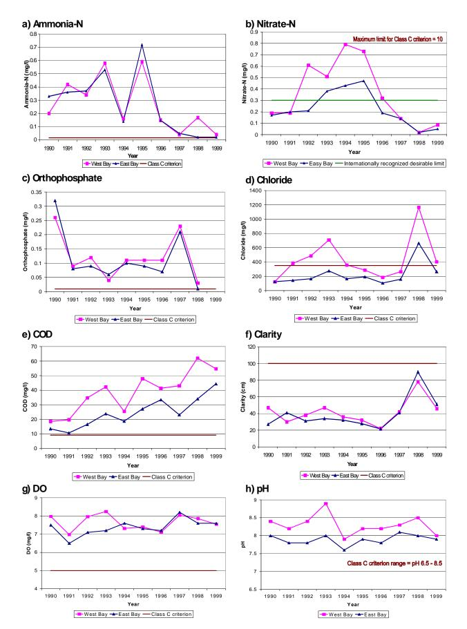
**Figure 4**. Concentrations of selected water quality parameters in the Laguna Lake, 1990-1999. These parameters have either exceeded or fallen below the criteria for Class C waters (Note: Barril's data = 1990-1996; LLDA data = 1997-1999).
