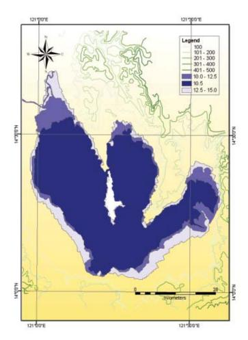
Figure 5.2. Interpolated water levels and digitized contour map. Source: LLDA IWRM Division.
