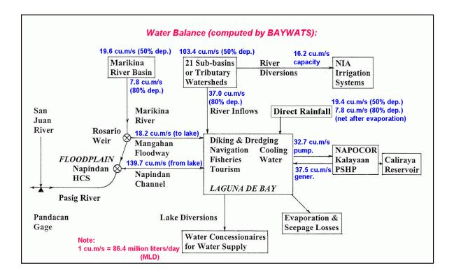
Figure 2.2. A water balance diagram of the Laguna de Bay for the selected mean lows and the 50 percent and 80 percent dependable river flows (NHRC 2000).
